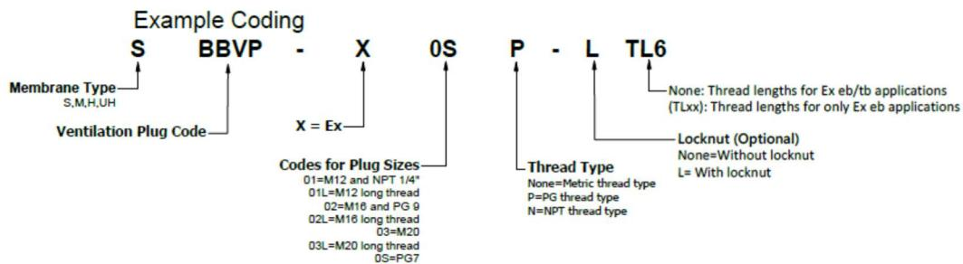
Note: (Thread Length) in the key code is mandatory for products having thread length different than the minimum TL for Ex eb/tb applications indicated in the assembly tables.
